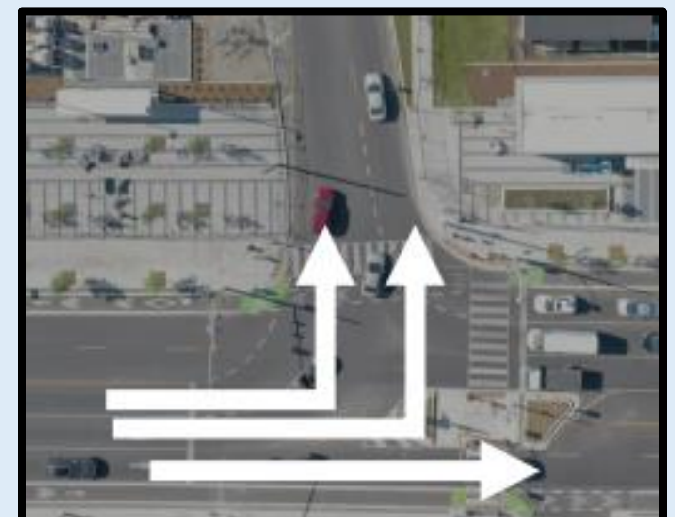
Phase 3B: North-South Pedestrian Signal NOT Activated
