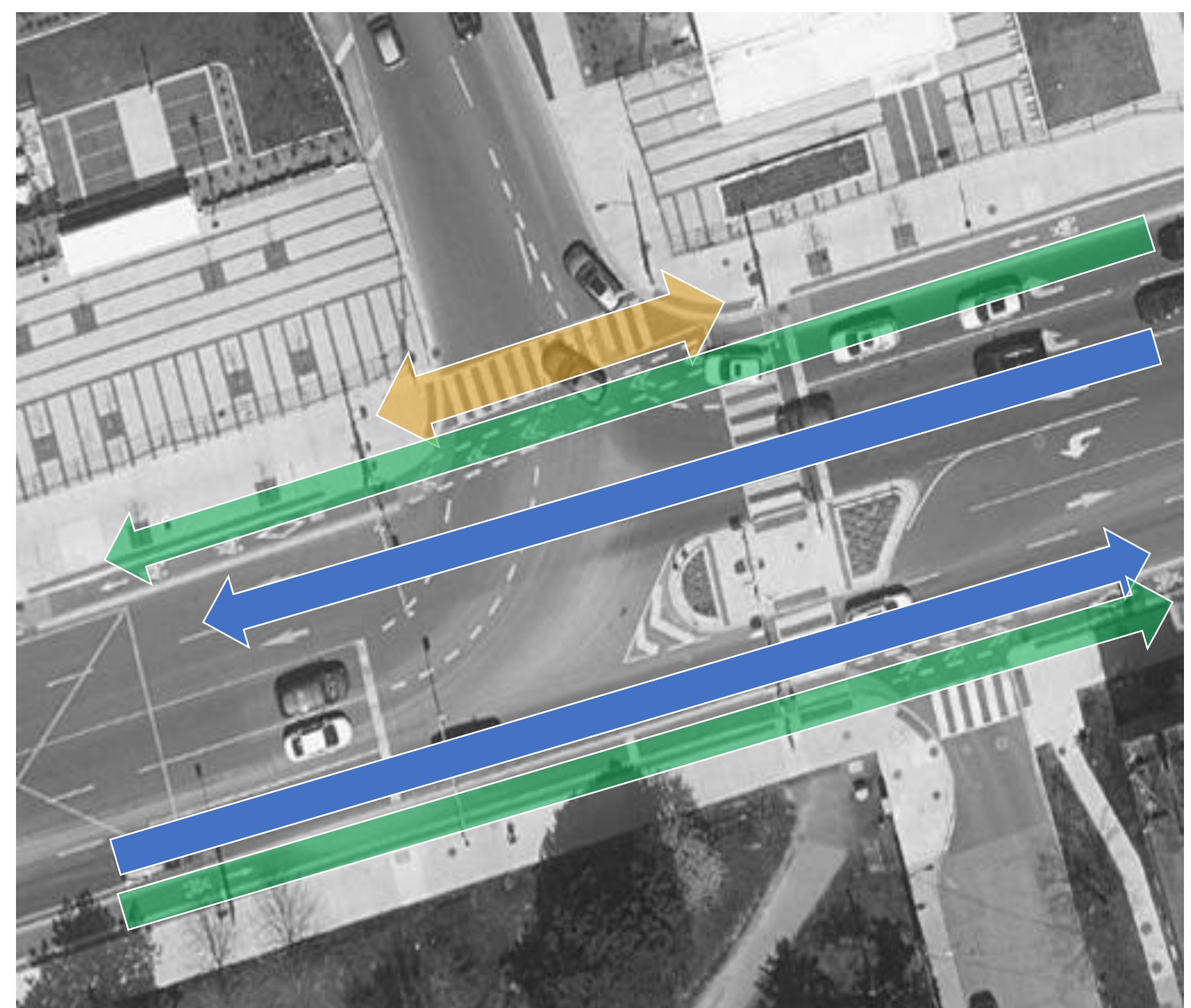
Permitted movements during the through-phase for traffic, demonstrating when pedestrians and people cycling can cross the on-ramp
